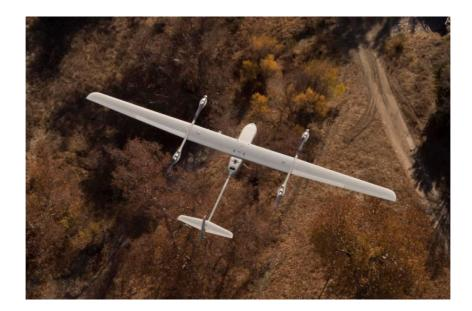
Weighing just over 20 kilogrammes with a 4.88 metre wingspan, the operatonionally proven STALKER drone is portable, vertical-launched and almost silent. It provides over eight hours of imaging capability and is able to cover around 60 miles. Image: Lockheed Martin UK
