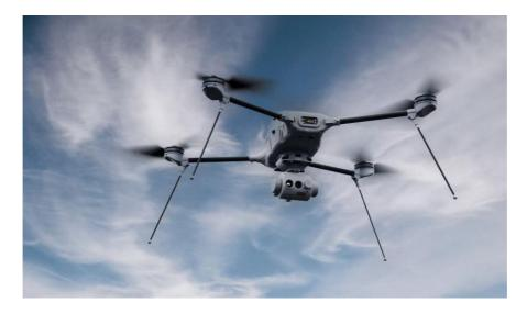
The foldable INDAGO 4 drone weighs less than 2.5 kilograms, can be carried in a soldier's backpack and deployed in just two minutes with a range of approximately eight miles. Image: Lockheed Martin UK.
