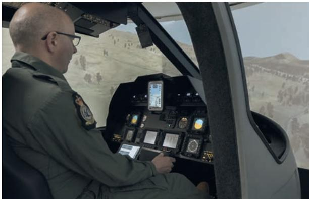
The Inzpire family of Targeted Fidelity Simulators deliver training solutions across a broad spectrum of capabilities and platforms including helicopters, fixed-wing aircraft, RPAS Ground Control Stations and Forward Air Controller environments. The simulators can be networked for linked or distributed operations in fully integrated synthetic environments. This enables multiple aircraft to train in formation at a single training facility, or to be networked across different locations.
